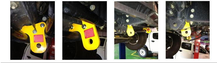
Ensure all supplied and specified components are used during the installation of tow recovery points, Failure to do so will significantly reduce the Working Load Limit (WLL) specified for each individual point, which can result in serious injury or death.
